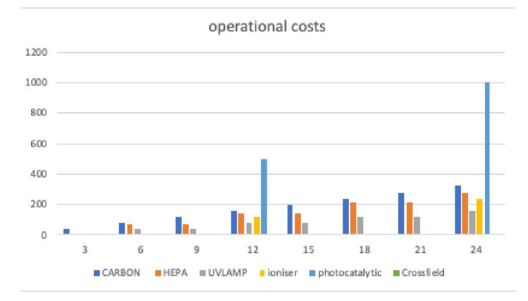
For the air purifiers with a filtering system combination, the operational cost must be considered the sum of a single system.
